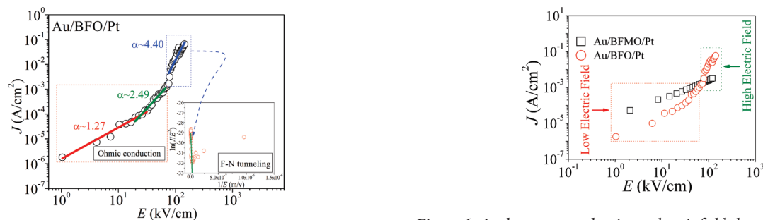
Figure 6. Leakage current density vs electric field characteristics of BFO and BFMO.
